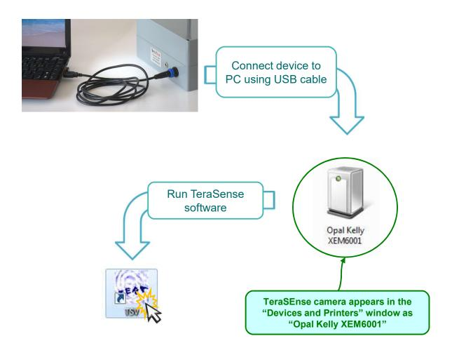
When connecting for the first time to a new PC you'll need to wait while Windows installing drivers for the device.
