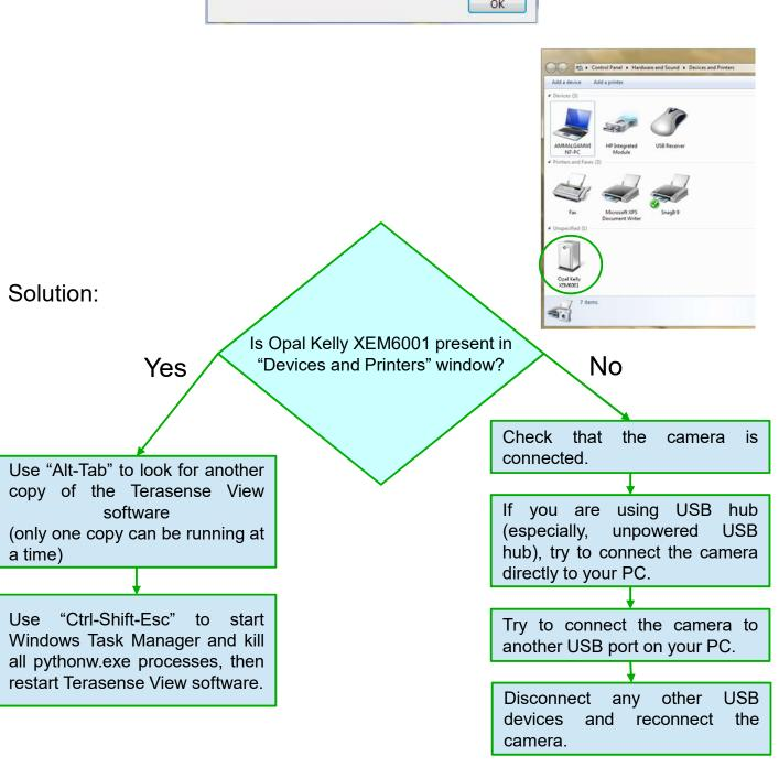
If the software have crashed (for example, due to the device being disconnected during the run) it may have left a zombie process, which would prevent new copy from running.
