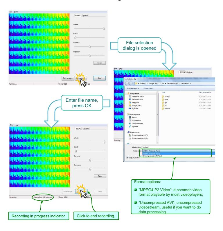
Generally, video is recorded at actual frame rate, but if it is less than 1 fps, frame rate of the video would be 1 fps.
